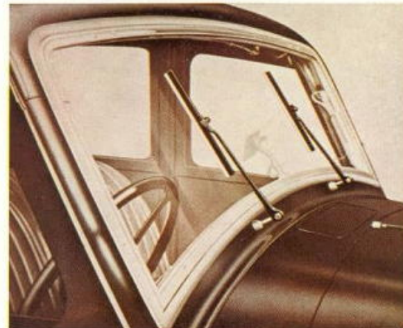
Twin windscreen wipers with a remote silent drive and with the passenger's arm independently controlled are provided to ensure clear vision in bad weather.
